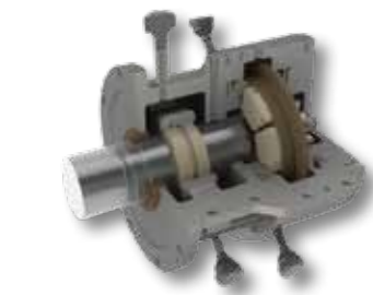
Above: Mechanical seal/labyrinth gland/impeller options/hydrodynamic bearings
